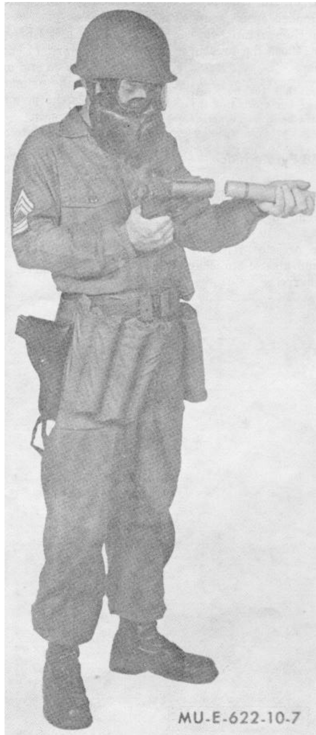
Figure 7. Loading cartridge into AN-M8 pyrotechnic pistol (typical).
